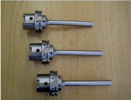
HSK-A100 x \varnothing 10 x \varnothing 23 x 260 Art.-Nr. 4004-422.00
